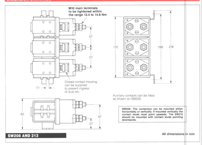
Pull-in voltages are approximately 60% and 66% of the rated voltage for intermittent and continuously rated types respectively.
