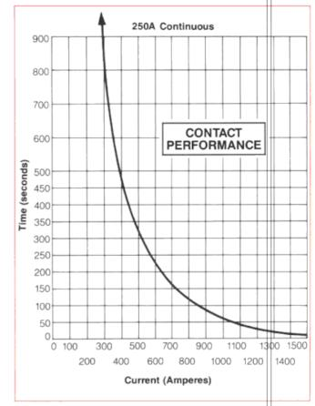
All the above figures should be used as a guide only. Some derating may be necessary according to type and application.
